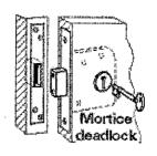
Use a heavy-duty strike plate with 3-inch screws to penetrate into a wooden doorframe.
